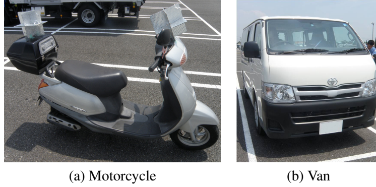
FIGURE 4.8: The vehicles used for the experiment. (a) A motorcycle with two corner reflectors attached on the front and the rear part. (b) A middle-sized van.
