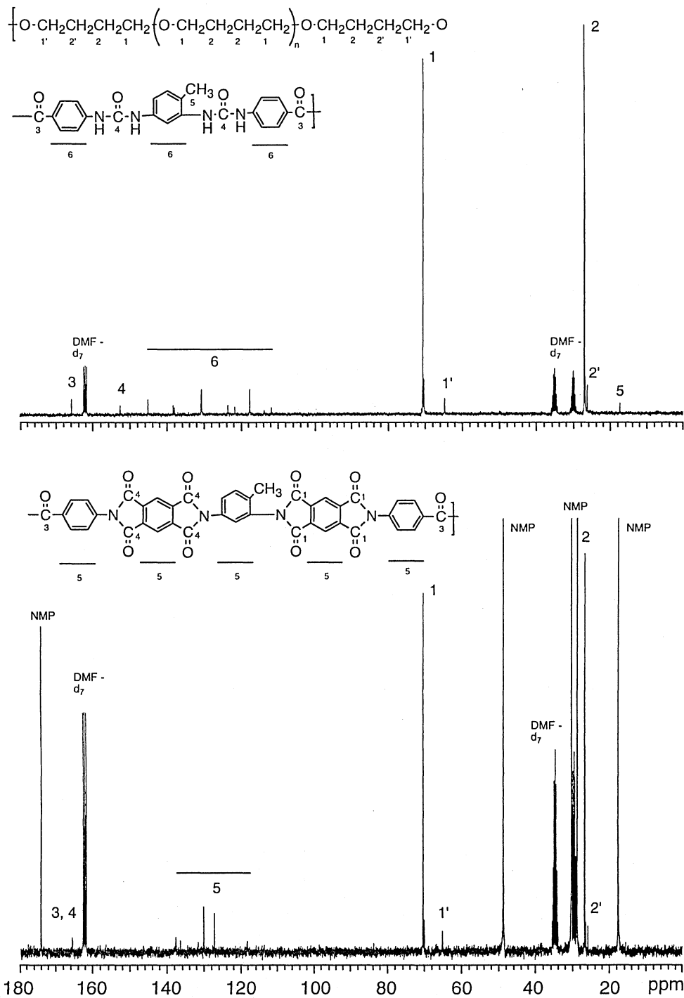
Fig. 23. ^{13}\text{C} - NMR spectra of 2,4-TDI based polyurea (1a) and IEP (2a) .
